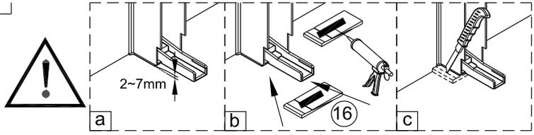
The setting wedge(No.16) will be needed if the profile is not level in 2-7mm.
